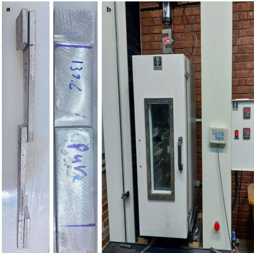
**Fig. 2.** Tensile test machine (a) and single-lap adhesive joint test samples (b)
